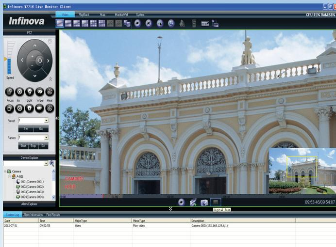
V2216 network video management software is a central management platform for all kinds of network video systems. It includes two versions: V2216 Professional and V2216 Enterprise. The former is suitable for medium surveillance installation and supports a maximum of 128 video inputs, while the latter is the most powerful software which is suitable for any large surveillance installation.
